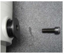
Remove #275118 Socket Head Cap Screw from #701015 Plug.
