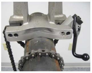
Both the #700993 Chain Hook, and the #700985 Chain Tension Block can be relocated to the opposite sides of the #700975 Frame if needed to fit in tight quarters.
