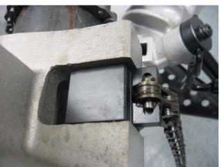
Once chain is hooked into the block, turn Handle #606742 in the clockwise direction to tighten frame to pipe.
