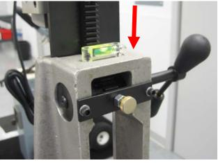
Place Plate #701063 (with drill attached) into the slot of frame. Turn Retractable Spring Plunger Knob #276899 90 degrees to lock feed handle.
