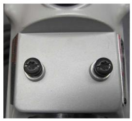
Replace handle screws back into threaded holes
