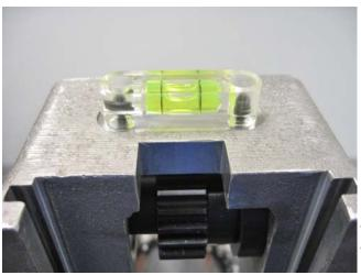
A bubble level is mounted on top of the frame for your convenience.
