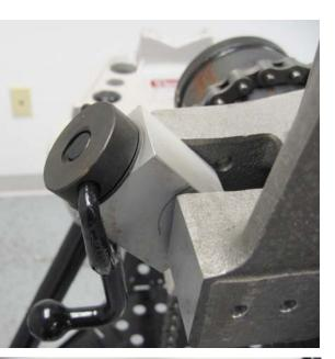
Turn Handle counter clockwise to lower Chain Screw threads.
