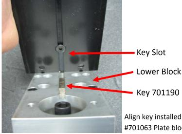
Align key installed on #700966 Lower Block to key slot on #701063 Plate block.
