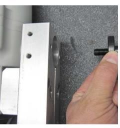
Install #275118 SHCS and #701014 Washer into the counter bored hole of #700996 Lower block. This will secure the block to the drill body
