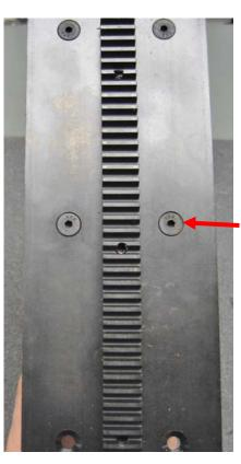
Install (4) #276888 ¼-20 Flat Head Cap Screws into Plate. Tighten all (4) screws using an allen key.
